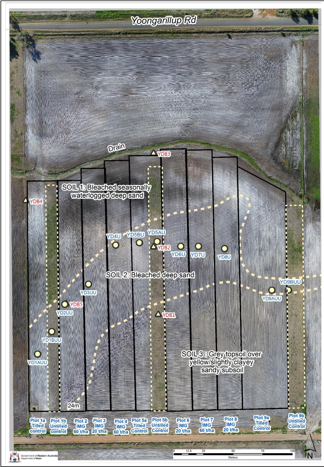
Figure 1: IMG experiment design on Yoongi Downs with monitoring sites (lysimeters labelled in blue, bores labelled in red).
