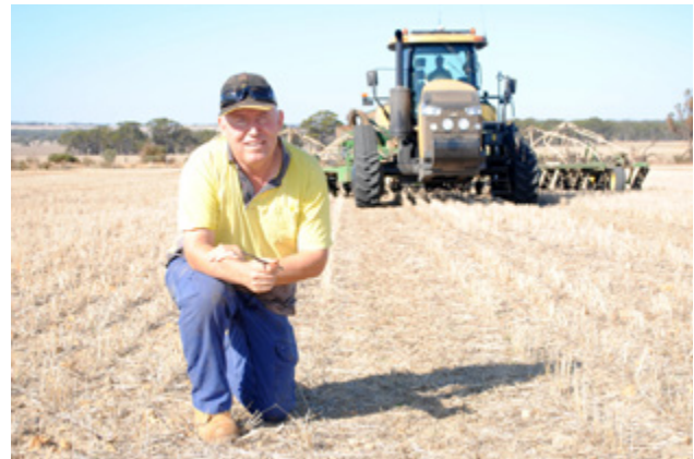
Gary Lang with his Cat® tractor on 3m wheel track centres, 11.9m wide John Deere Conserva Pak™ air seeder and Simplicity bin. PHOTO: GRDC
