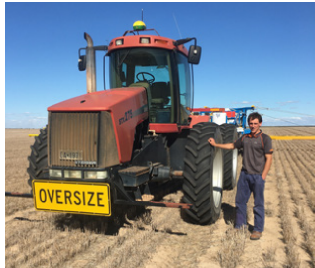
Carnamah grower Avon Rayner uses a Case IH STX275 tractor to pull a 31.8m Sonic boomspray in his controlled traffic system. PHOTO: Peter Rayner
